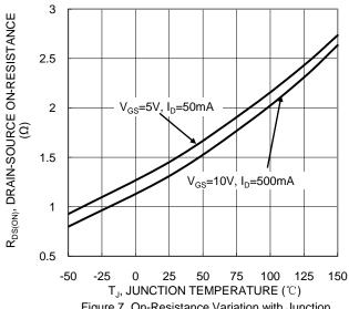
Figure 7. On-Resistance Variation with Junction Temperature
