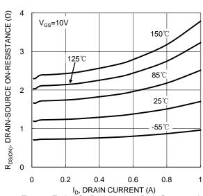
Figure 3. Typical On-Resistance vs. Drain Current and
