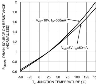
Figure 6. On-Resistance Variation with Junction Temperature
