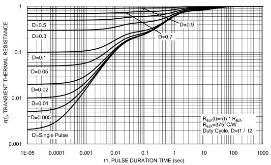
Figure 13. Transient Thermal Resistance
